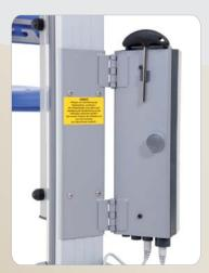
The battery can be removed at the side for narrow doors.
